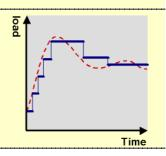
The tab« filter simulation » allows you to select and set the 3 successive filtering levels of eNod3 before viewing their effect on the signal.
