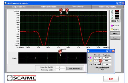
In our example, the weighing cycle is triggered by a logic input. We thus positioning the cursor **(B)** at the state change of the input **(C)**.
