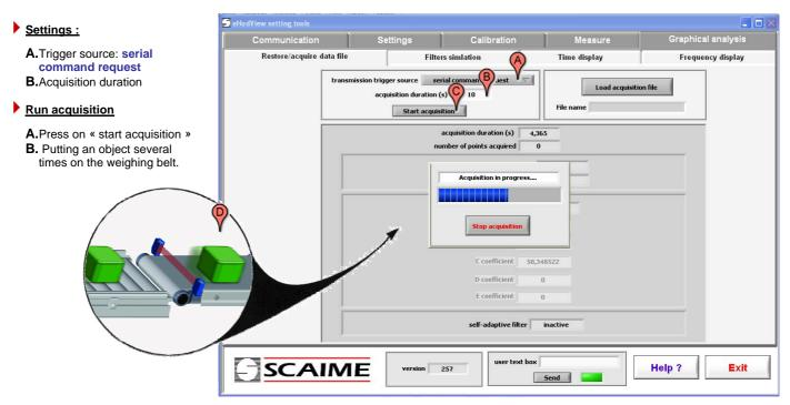
Now, you are ready to analyse the acquisition signal and optimize the digital filter settings.
