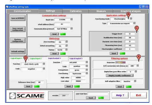
We can now check the proper functioning of the dynamic weighing cycle by using the "Measure" tab.
