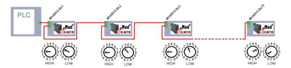
PROFINET IO network and names of **eNod4-T** stations in factory configuration. Only rotary switches have been reconfigured.
