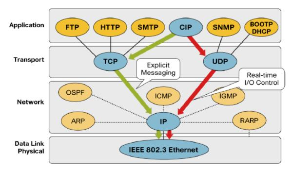
By using TCP/IP, EtherNet/IP is able to send explicit messages, which are used to perform **client-server** type transactions between nodes. Nodes must interpret each message, execute the requested task and generate responses. Uploading and downloading of configuration data like setpoints and applicative parameters uses **explicit** (or Class 3) messaging.
