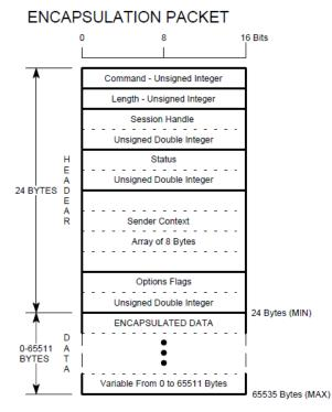
For any data to exchange, the encapsulated data format is **most significant bit (MSB) transmitted first.**Access to the object model of a device is controlled by one of two objects: the Connection Manager, and the UnConnected Message Manager (**UCMM**). We have already stated that EtherNet/IP is a connection-based network
