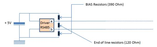
The BIAS resistors you need to install could be between 390 Ohm and 4.7 kOhm depending of resistors already installed on the driver. This modification should be done on the master itself. The high polarization must be done with the driver's 5V.
