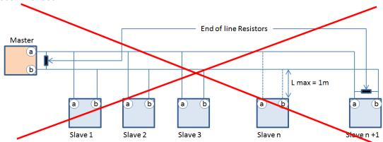
However if a node must be added in an existing network and it cannot be made otherwise, the node must be connected with the primary network by a cable. This cable must have a maximum length of 1m and an impedance of 120  $\Omega$  max:
