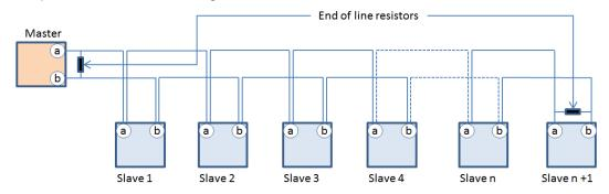
Be careful the following wiring is not equivalent to the precedent one: This second one is not recommended:
