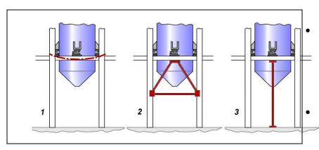
Figure 1 shows how a support beam can deflect when a weigh module is mounted at mid-span. If this type of arrangement cannot be avoided, you should reinforce the support beams to minimize deflection.
