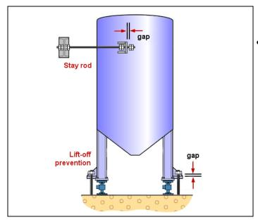
Stay rods are used to limit a tank's horizontal movement so that it will not tip or rotate. They should be positioned at or above the centre of gravity of the full tank.
