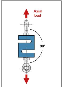
When utilizing tension cells for vessel weighing:
