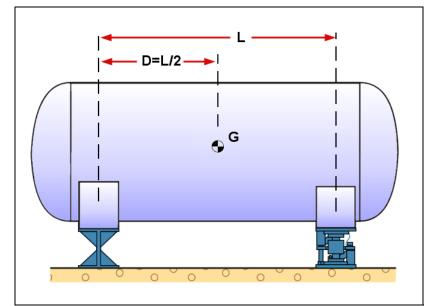
In fact, not the weight, but the force is measured by the load cell. The force on the load cell(s) can be calculated by:
