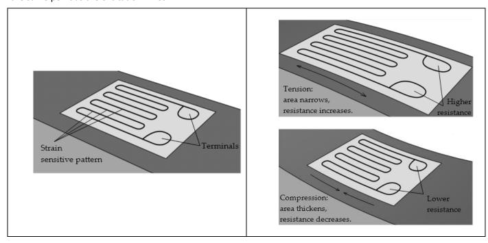
If the gages within a load cell are connected in a balanced Wheatstone Bridge circuit, and are excited by a source of AC or DC voltage, the transducer will produce an electrical output which is a direct linear function of the excitation voltage.
