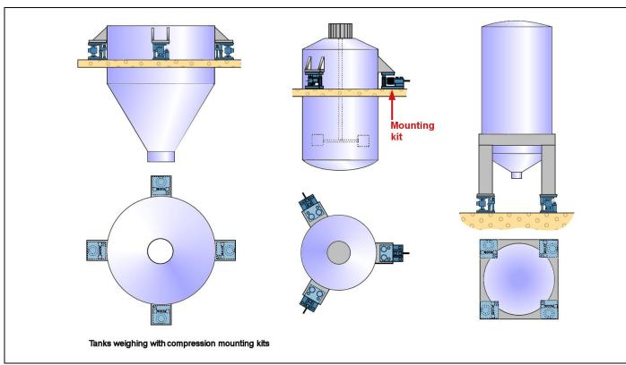
To help load cell mounting, SCAIME offers compression mounting kits especially designed for tank weighing. A typical compression mounting kit includes a top plate (which receives the load), and base plate (which is bolted to the floor or other support surface). Some kits provide also additional devices (see data sheet) as:
