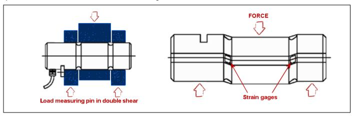
Load measuring pins are designed for many diverse applications as direct replacements for clevis or pivot pins. They have many advantages over other load sensors in that they do not normally require any change to the mechanical structure being monitored.
