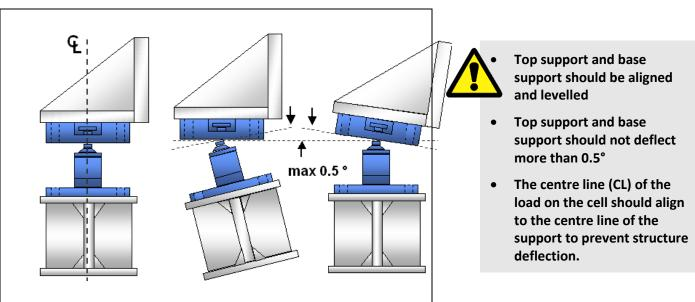
The weight error will increase with the angle at which the support is leaning:
